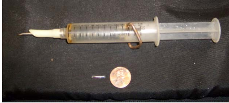
Figure 2.3: Picture of a PIT-tagging needle and PIT-tag in relation to a penny.
